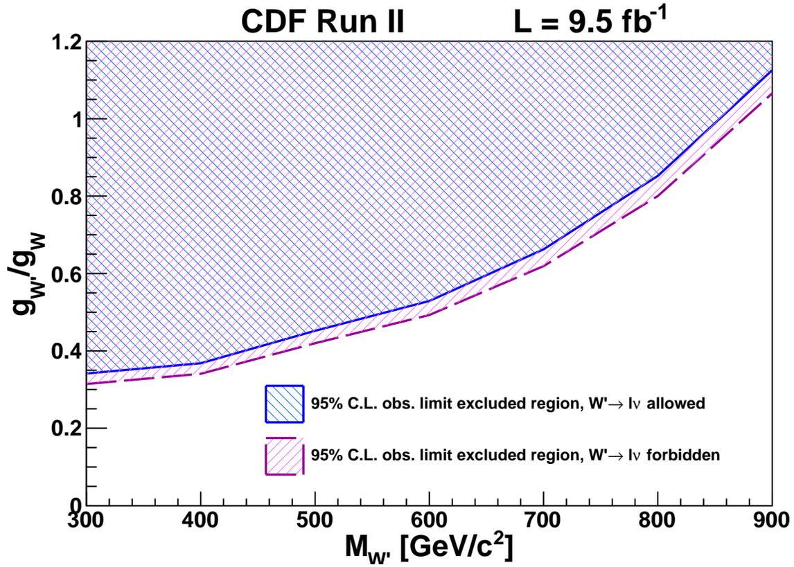
FIG. 4. Observed 95% C.L. limits on the coupling strength of a right-handed  $W'$  compared to the SM  $W$  boson coupling,  $g_{W'}/g_{SM}$ , as a function of  $M_{W'}$  in cases where the leptonic decay mode  $W' \rightarrow \ell\nu$  is allowed or forbidden. The patterned region above each line is excluded.
